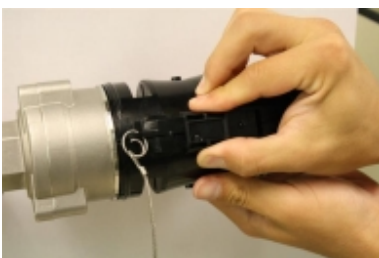
Figure 19 Remove Environmental Guard
