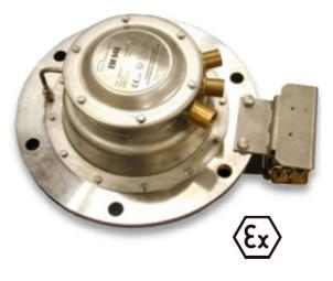
The EM940 Radar employs advanced smart sensor technology packaged with a planar antenna. The radar beam is shaped electronically without the use of additional mechanical parts like a lens or horn as seen in traditional radar type level sensors. The integrated IG (inert gas) pressure transmitter offers added measurement parameters from a single instrument.
